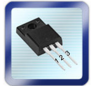
T0220 Full-PAK Isolated (T0-220) 1=Gate, 2=Drain, 3=Source
